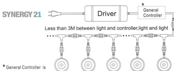
\* General Controller is used to control the RGB light.
