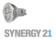
GU10 base 4x1Watt LEDs ALU housing Operating voltage 85-265V Power consumption: 4 W Lumem: -Kelvin 940nm Infrared Beam angle 60° Dimmable: no DxH: 50mm\*60mm Can be used as a replacement for conventional halogen mirror lamps.
